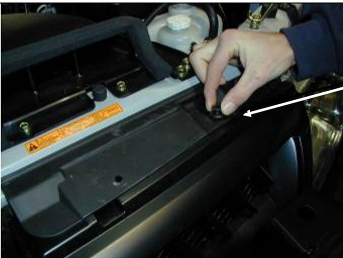
3. With all of the plastic plugs, two screws and two bolts removed from the lower bumper bar , the grille and grille cover must be removed. There are three plastic plugs that hold the cover in place, remove these as previously described above.
