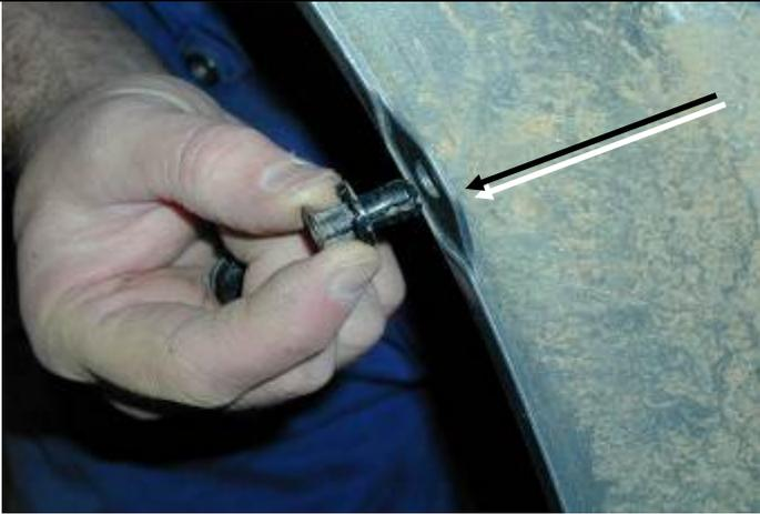
1. To remove the bumper bar from the vehicle , remove the 3 plastic plugs that hold the plastic guard liner to the bumper bar on each side using a small flat bladed screw driver .
