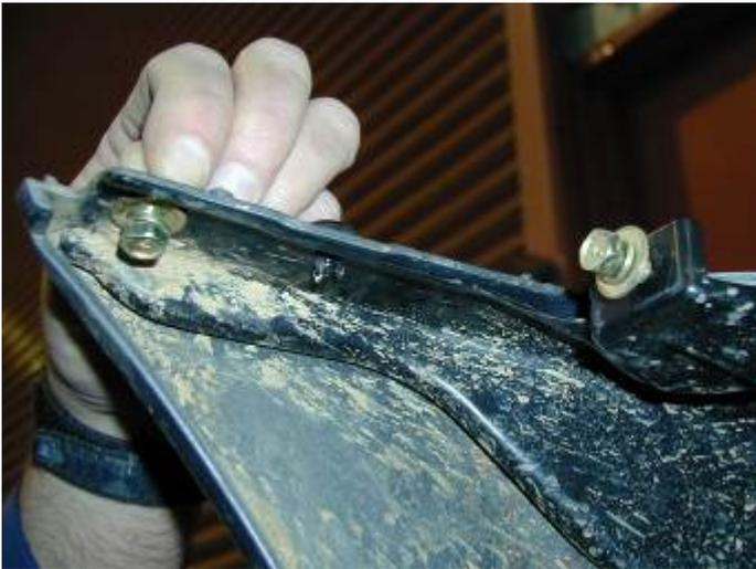
2. Using a Philips head screw driver remove the vertical screw on the out board top edge of the bumper bar ( this screw and following bolt are accessed from the wheel arch area ) . Using a 10mm socket remove the horizontal bolt , as shown in the photo .
