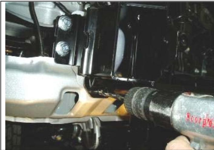
7. Drill Dia 10.5 pinning hole in lower flange of mount bracket into the vehicle crossmember
