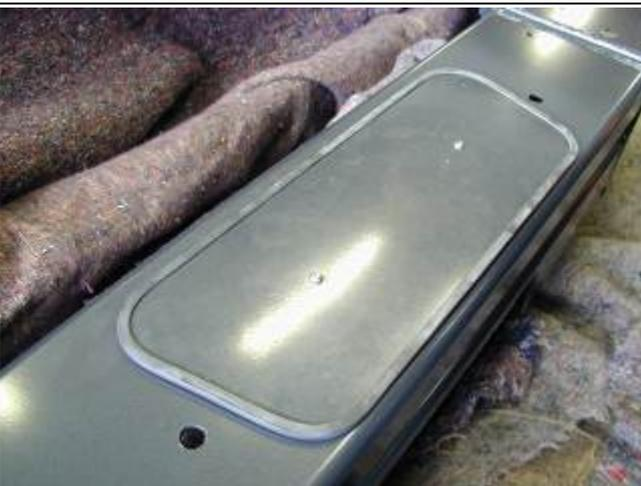
18. Where a **WINCH IS NOT FITTED** :- Wrap the rubber extrusion around winch cover.
